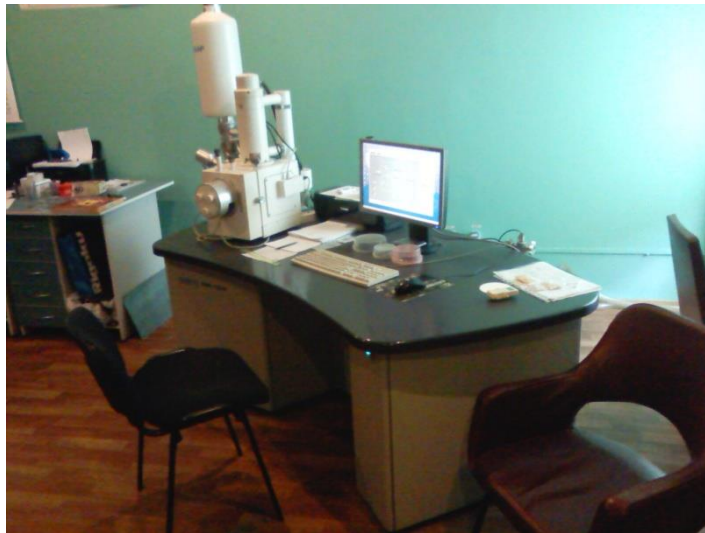
Picture 1.5 - Scanning electron microscope REM-106I of Selmi (Ukraine)
