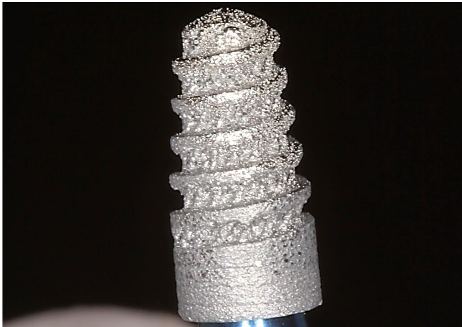
Pic. 3. Titanium implant with double-layered mesh-like surface macrostructure.
