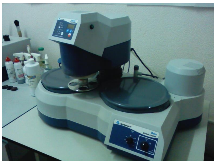
Picture 1.4 - Automatic grinding and polishing machine GP beta by Buehler (Germany)
